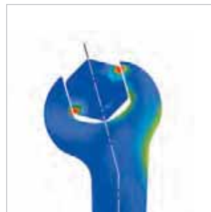
2 Load zones in spanners by STAHLWILLE
