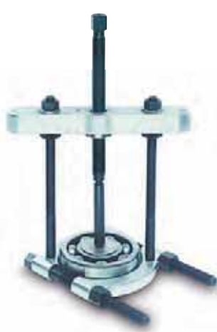
Separating fixture in use for removing ball bearings
